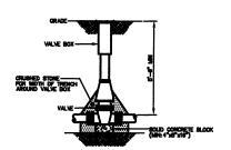
1. VALVE BOX SHALL BE CENTERED ON VALVE AND SET ON COMPACTED BACKFLL 2. VALVE SHALL NOT SUPPORT VALVE BOX. VALVE SCALE: NOT TO SCALE
