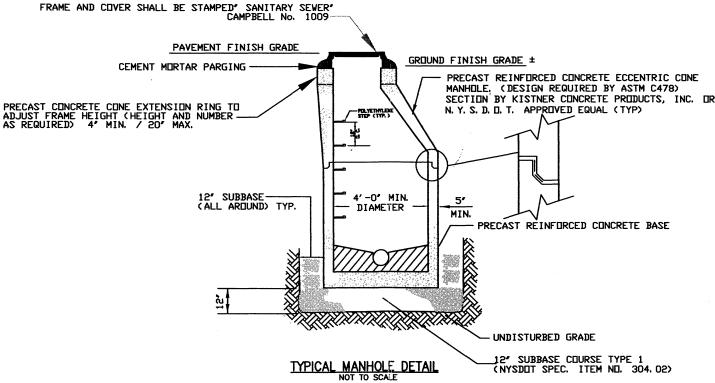
NOTES: PRECAST CONCRETE SUPPLIERS SHALL BE ON THE NYSDOT APPROVED LIST PLUG ALL LIFTING HOLES WITH CEMENT MORTAR PRECAST REINFURCED CUNCRETE MANHULE SECTIONS 4000 P.S. I. AT 28 DAYS, 5% AIR ENTRAINED, ASTM-A497 REINFURCING STEEL ASTM A615-A497 AASHTO H-20 LOADING WITH 30% IMPACT AND 30 P. S. F. SOIL PRESSURE
