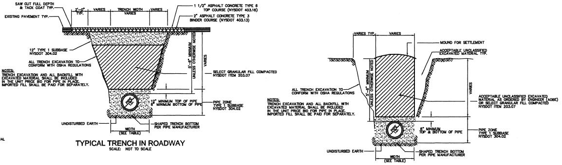
TYPICAL TRENCH IN EARTH OR ROCK SCALE: NOT TO SCALE
